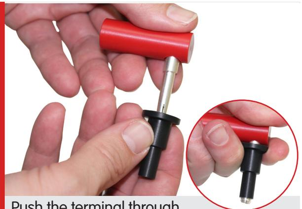
Push the terminal through the spring and sleeve.
