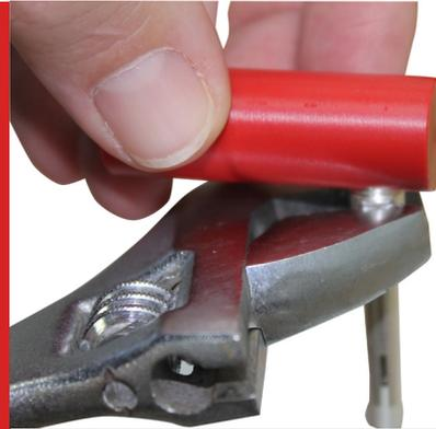
Use a wrench or spanner to snug tighten. Ensure the Smartfuse welding terminal is connected to the red lead, and the standard welding terminal is connected to the black lead.
