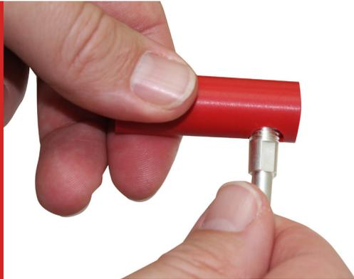
Tighten the welding terminal into the threaded lead connector, initially by hand.
