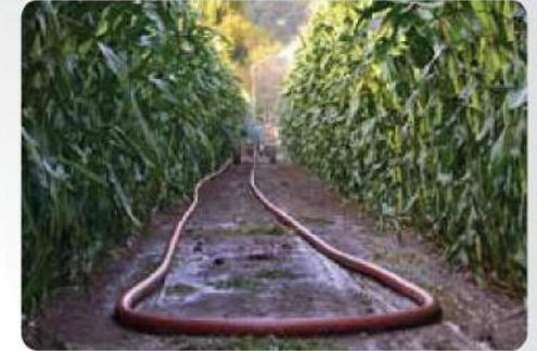
IrriCruiser is a new generation soft hose travelling irrigator designed to provide energy efficiency and highest performance. The turbine provides high torque to pull the irrigator and hose along the steel cable even in tough condition.
