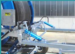
▶ Hydraulic pump and lifting system for trolley
